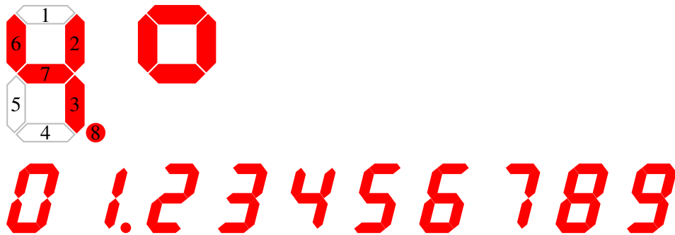
Figure 86: A customizable seven-segment display showing the numbered segments, a custom shape, and the numerals from 0 to 9 [Sevenssegment.m4].
